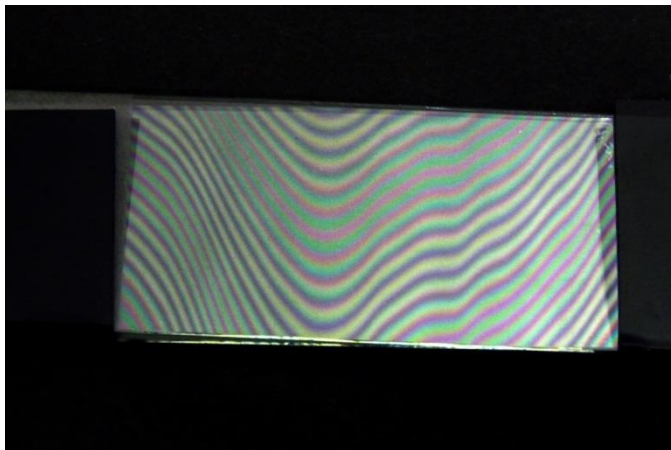
Lay a glass slide on another, due to the sandwiched air space
